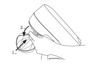
**NOTE** Be sure the attachment is locked firmly in place.
