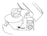
**NOTE** The bowl should feel firm with no movement. **5**. Lower the mixer head with the selected mixing attachment in place into the mixing bowl. Press the 'head release' button to unlock it from its position and ease the mixer head down (Figure 4).
