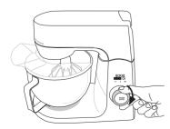
**6**. When mixing is complete, turn the speed control dial anti-clockwise to the '0' position (Figure 7) and unplug the cord from the power outlet.
