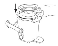
IMPORTANT: Ensure that the card disc protecting the Double Sieve filter basket blades is removed before use.
